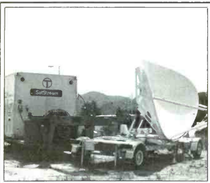
A new, small portable earth station used by NBC on Cyprus. This Ku-band (12 to 14 GHz) equipment was made by McMichael and airlifted to Cyprus. The receiving station was the Madley Earth Station in England (operated by British Telecom).
