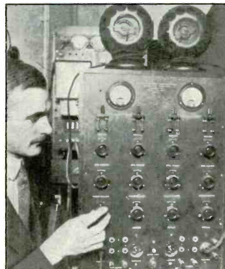
WNAC developed a 2-microphone mixing method used for music reproduction. In this 1923 photo, CE Sam Curtis shows off this device. One microphone was specifically designed to pick up the bass tones normally lost in early broadcasting.
