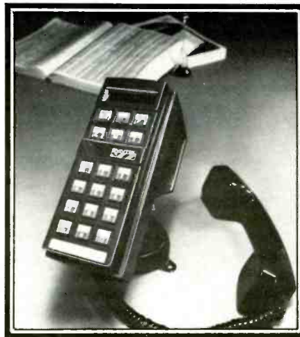
This mobile phone control head manufactured by Antenna Specialists Co. allows 800 MHz trunked mobile radios to be utilized as mobile telephones through repeater interconnects.
