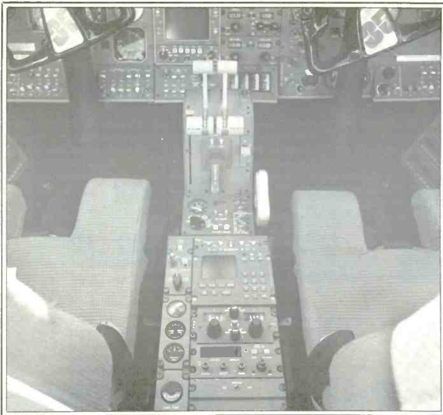
Aircraft flying international routes can communicate on frequencies normally active during skyjacking. The HF transceiver in this Gates Learjet 35 is mounted in the center console at the bottom of the photo.
