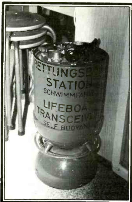
Teun Feldman of the Netherlands snapped this photo of a floating emergency radio used by large ocean-going vessels. It probably operates on 500 and 8364 kHz CW as well as 2182 kHz and other voice frequencies.
