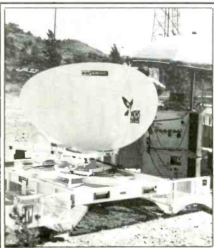
The Ku-band transportable earth station was flown in by a cargo aircraft called a Belfast (similar to a U.S. C-130). It was set up for full operation in less than 12 hours by its crew of three technicians.
